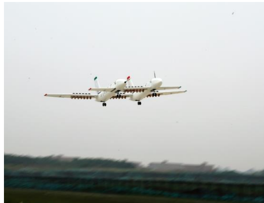
Figure 15 – Flight testing of the DEP demonstrator.
