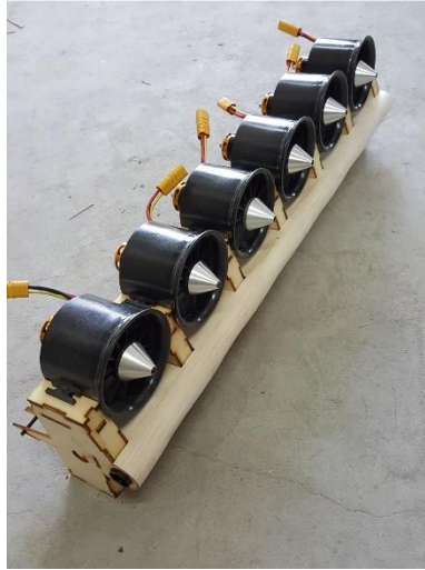
Figure 5 – Flap with EDFs mounted.
