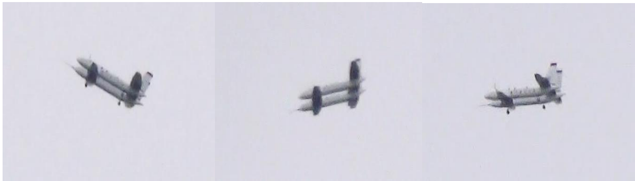
Figure 18 –Pitch control and response snapshots of the DEP demonstrator (from left to right).
