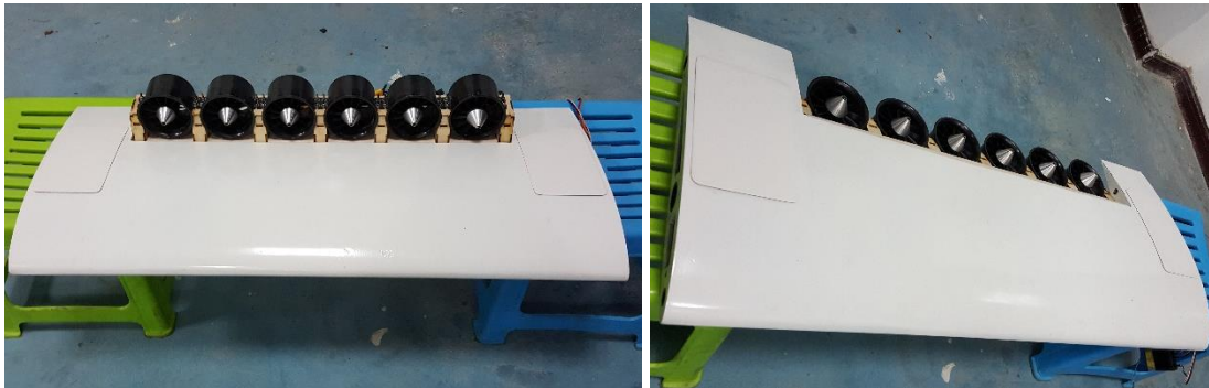
Figure 6 – Wing with the DEP system installed.
