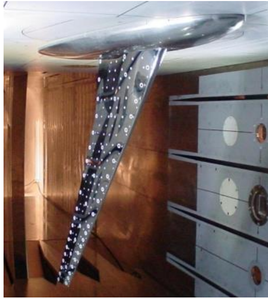
Figure 8 – Wind tunnel model of CRM configuration[22].
