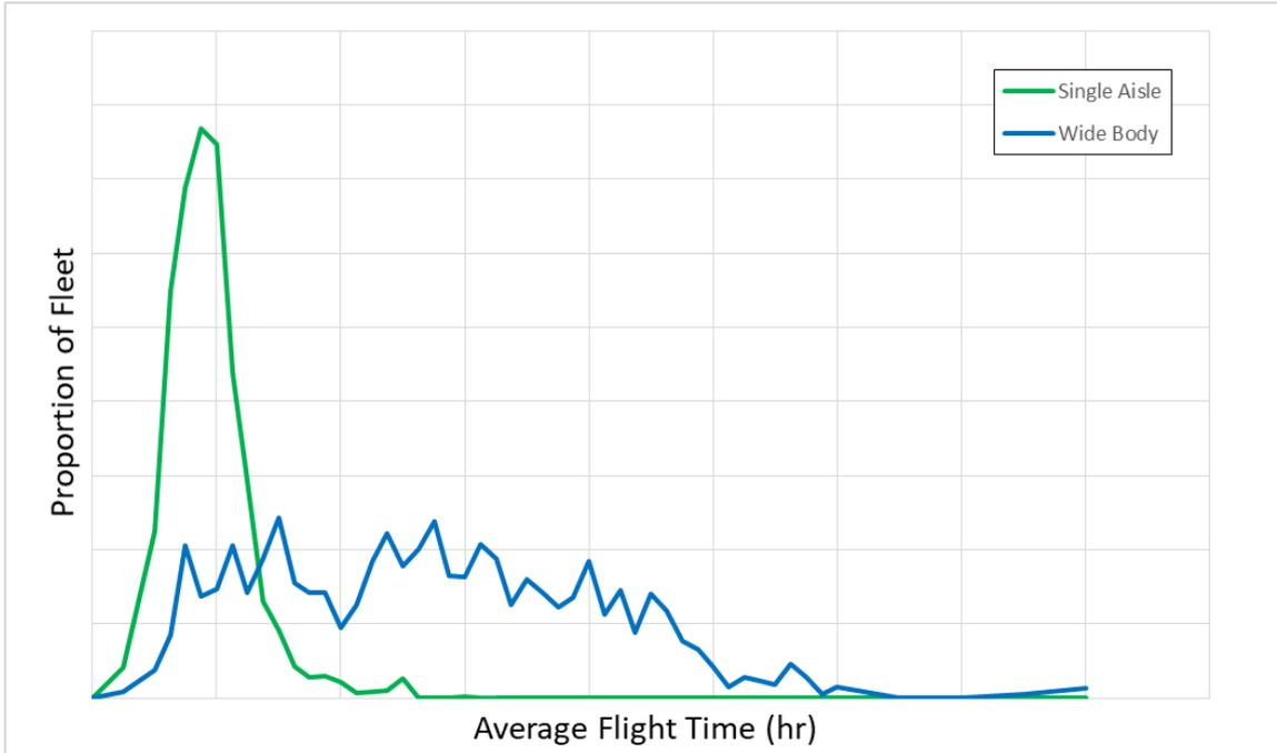
Figure 3 - Fleet operation for Single Aisle and Wide Body aircraft
