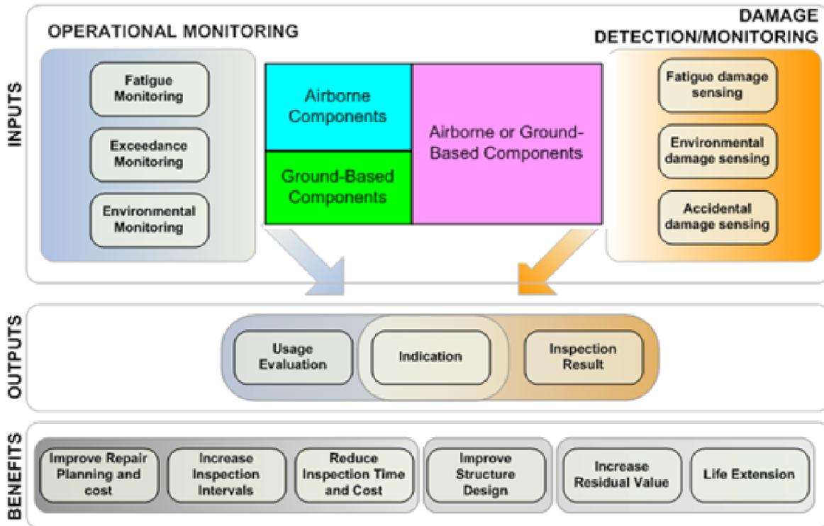
Figure 1 - Structural Health Monitoring following ARP 6461 [2]
