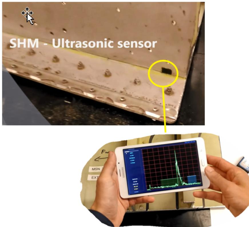
Figure 5 - Example of on-ground sensor interrogation
