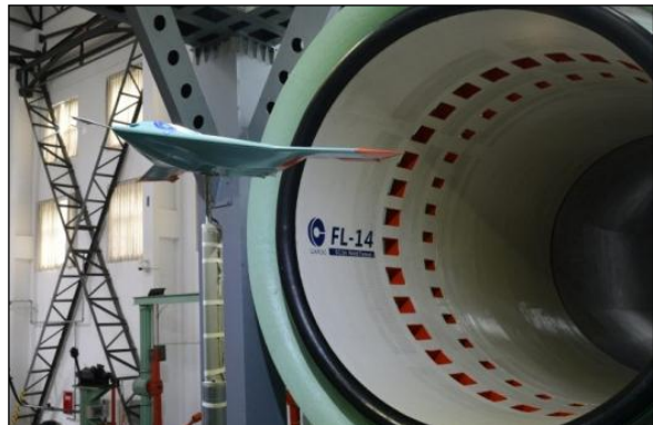
Figure 9 – Virtual flight test of the BWB model.
