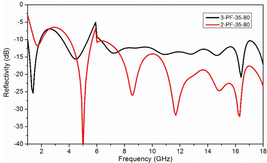
Figure 5 the influence of the cell dimension on the reflectivity of MAHCMs
