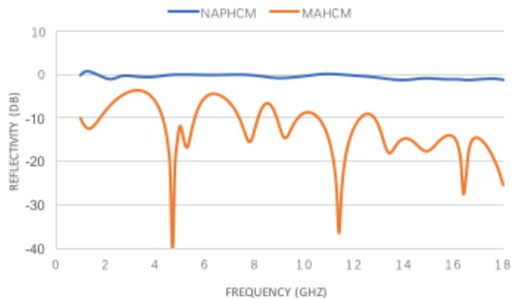
Figure 1 The reflectivity of NAPHCM and MAHCM
