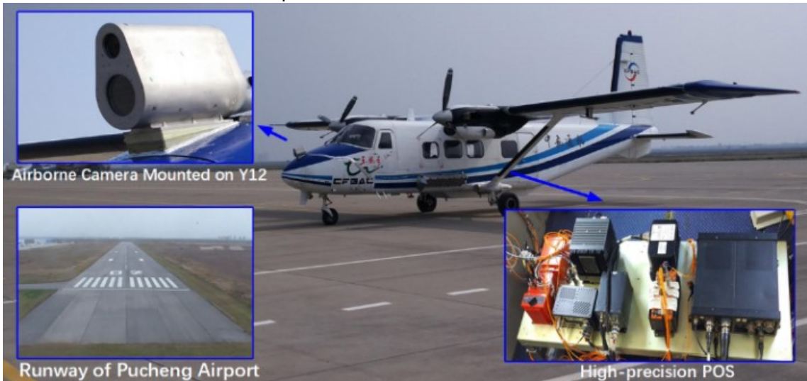
Figure 8 – Instruments mounted by Y12 and runway for data acquisition
