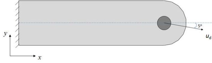
Figure 2 – Demonstration of boundary conditions and external load.
