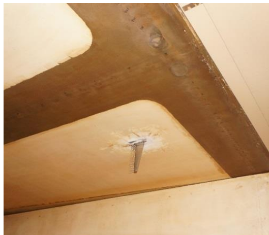
Figure 2 – Rake mounted on the nozzle upper wall.
