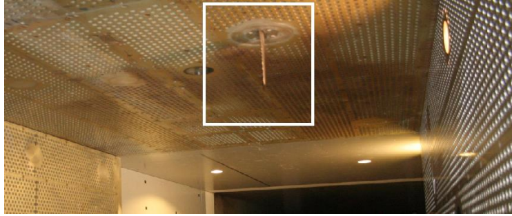
Figure 3 – Rake mounted on the upper wall of test section #2. Similar rake was mounted on the side wall of test section #1.
