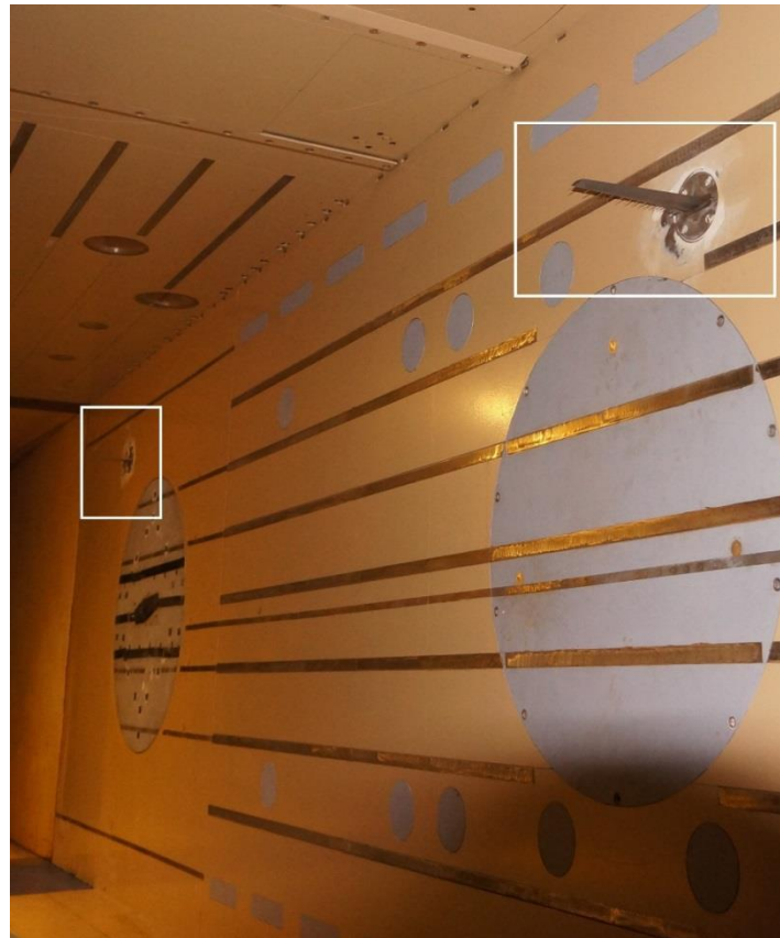
Figure 4 – Two rakes mounted on the side wall of test section #3.
