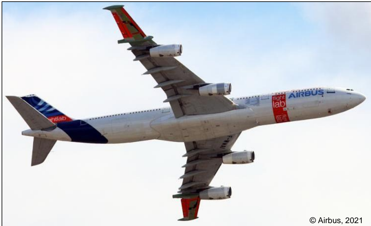
Figure 1 – BLADE aircraft, with the NLF panels apparent outboard of the outer engines.
