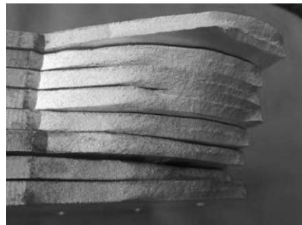
b) Characteristics of fatigue fracture appearance
