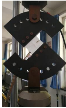
Figure 4 - Experimental setup of CTS specimen under mixed-mode loading
