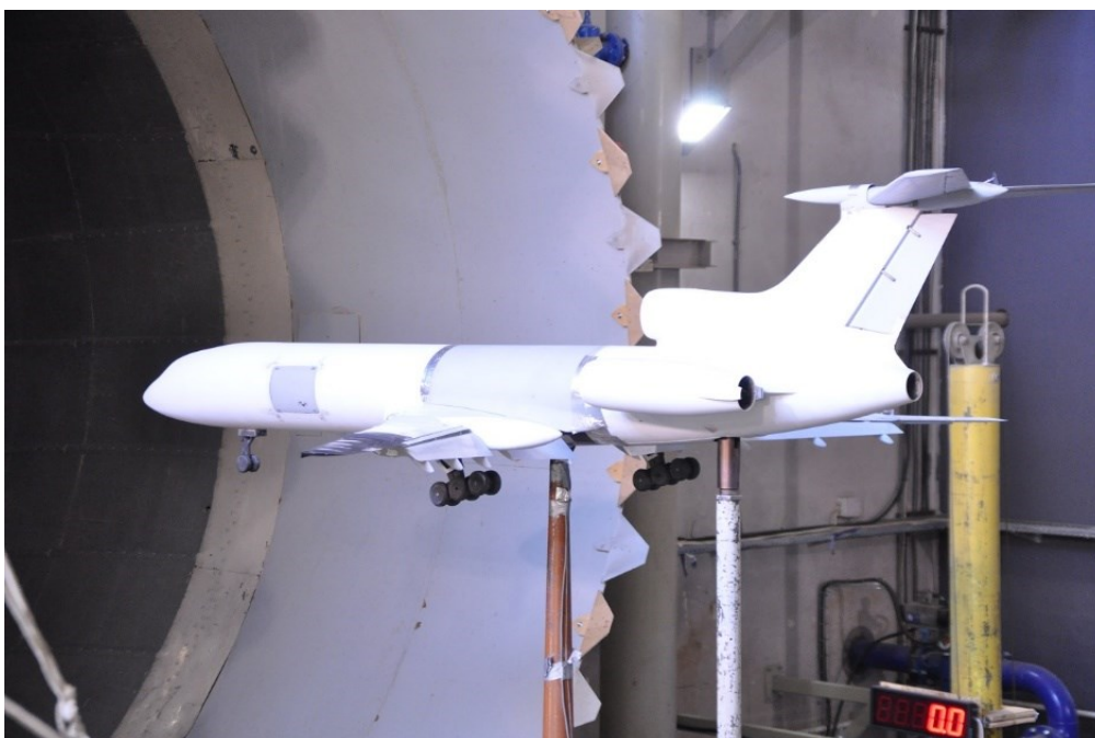
Figure 1 – The Tu-154M aircraft model in low speed wind tunnel T-3.
