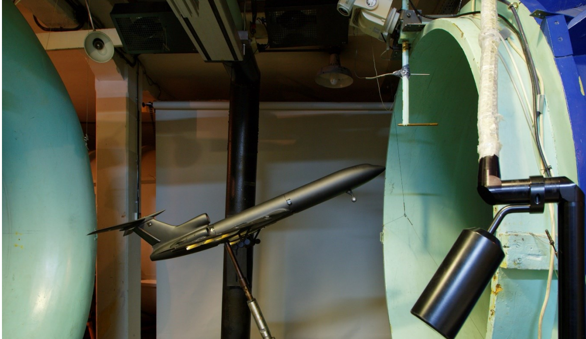
Figure 2 – The Tu-154M aircraft model in low speed wind tunnel T-1.
