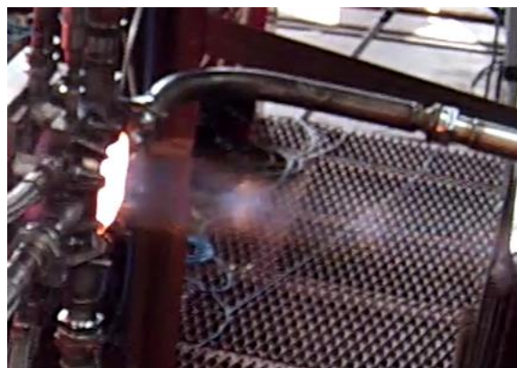
Figure 3 – Photo of thermal radiation shock waves in high temperature test jet.
