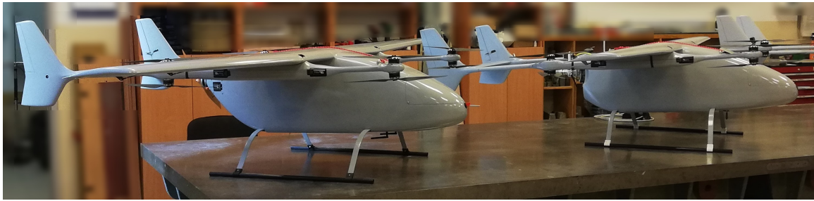
Figure 2 – Two PW Chimera: full electric (left), mixed propulsion (right)
