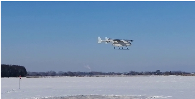
Figure 19 – PW Chimera - prototype - hover test (January 2021)
