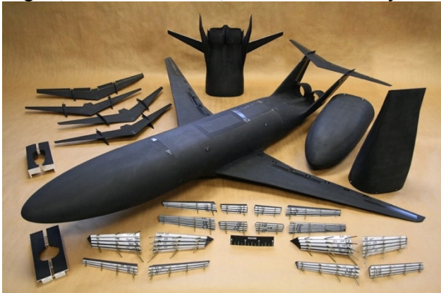
Fig. 22. 5%-scale D8 wind tunnel model. This model was used in the Aug 2016 D8 configuration wind tunnel test conducted at the 12-ft LST at NASA LaRC. Shown is the nominal OML (fully assembled), alternate tails (low-mounted horizontal tail, tail-off), alternate nose, and control surface [29]
