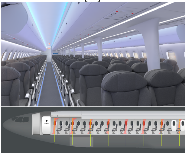
Fig. 15. D8 Central Structural Elements
