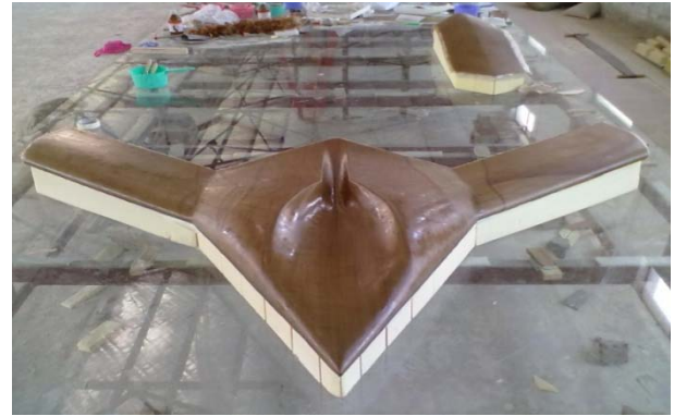
Fig.18 Demonstrator Glass Fiber Composite Skin
