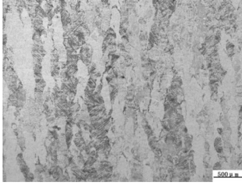
(a) Longitudinal section through columnar grains of the prior-β phase in the X-Z plane
