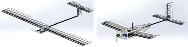
Fig. 7. Endurance-focused and agility-focused fixed-wing baselines
