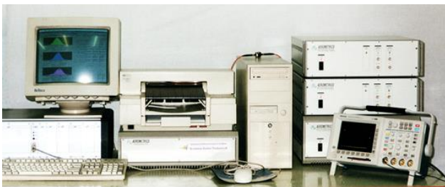
Fig. 3. 3-LDV Analysers, PDPA Analyser, Traverse Programmer, Computer with Printer, Oscilloscope
