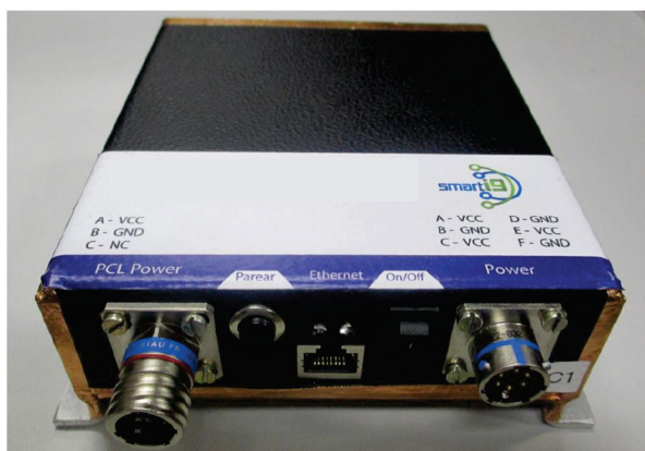
Fig. 5 The prototype of the PLC modem.
