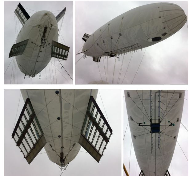
Fig. 8 Tether system attached to the airship.
