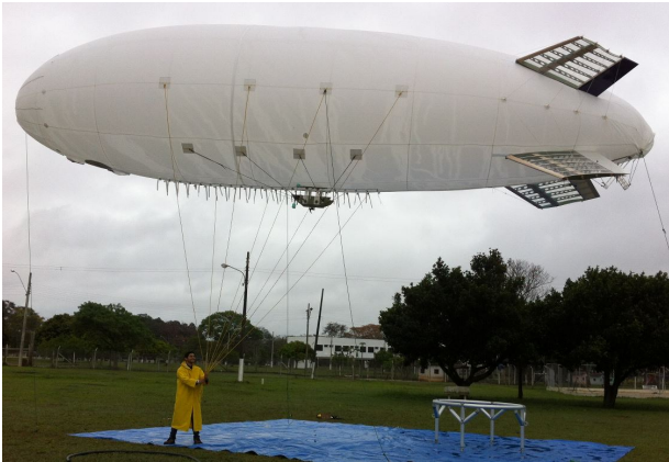
Fig. 10 Tethered airship prototype.
