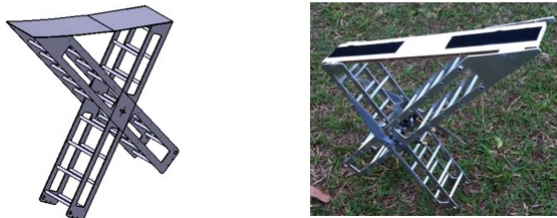
Fig. 7 Tail engine support.
