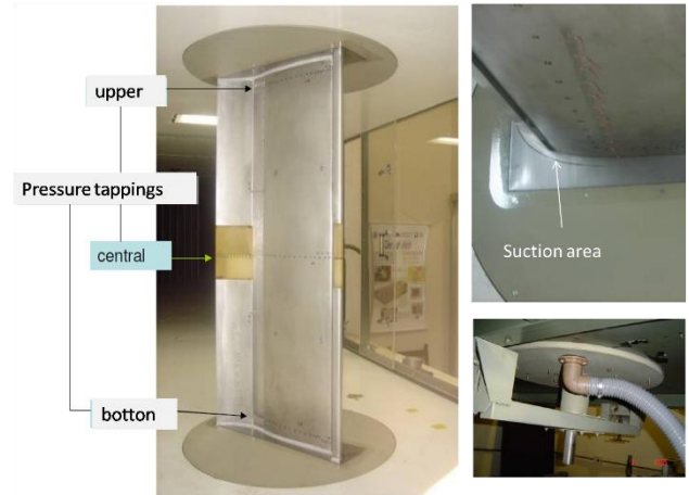
Fig. 3 High-lift experimental set-up with wind tunnel wall boundary layer suction.
