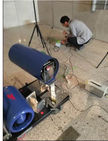
Fig.5 Noise reduction measurement system in reverberation chamber
