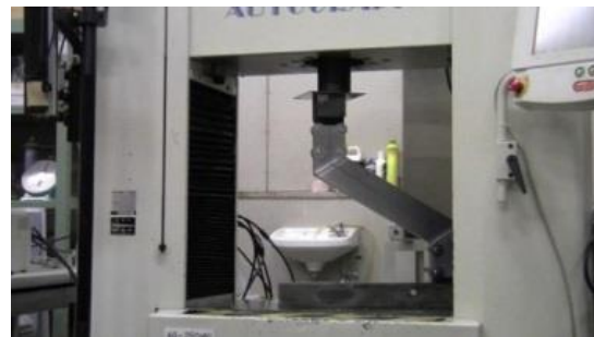
Fig.10 Strength test of the crushable frame
