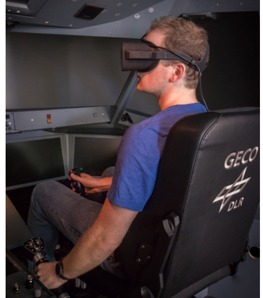
Fig. 3 – Simulator setup with virtual reality goggles and active force feedback helicopter controls.
