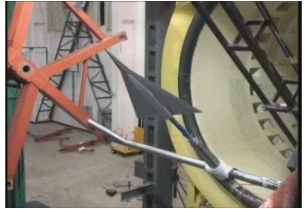
Fig. 13. Free to Roll Test for a Double Delta Wing
