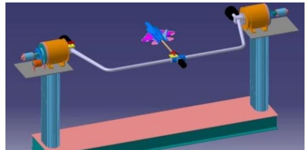
Fig. 4. Two DOF Dynamic Test Rig in Ø 3.2m W.T.
