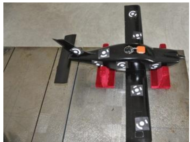
Fig. 17. Model Attitude Measurement
