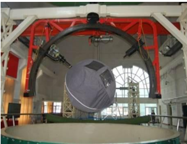
Fig. 15. Damping Ball for Rotary Balance Test
