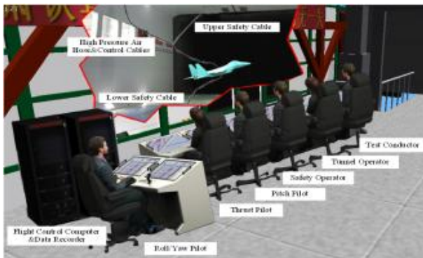
Fig. 19. Free Flight Test with Power
