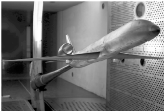
Fig 5: The aerodynamic model of low-sweep wing (LSW-2) aircraft with over-wing nacelles
