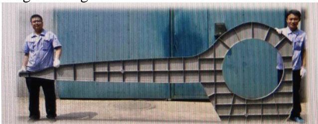
Fig.2. Half part of an airframe manufactured via AM
