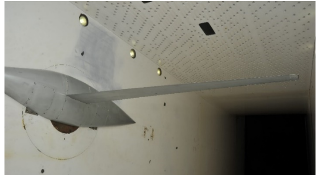
Fig.11 Model arrangement in the wind tunnel.
