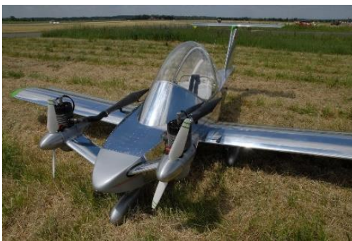
Fig. 10. Cri-Cri, the World smallest twin engine manned aircraft designed by French Colomban ( https://en.wikipedia.org/wiki/Colomban_Cri-cri )
