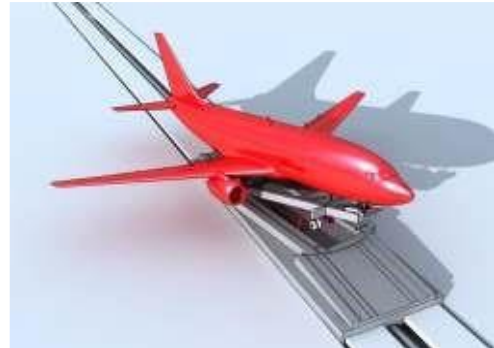
Fig. 8. Take-off and landing assisted by magnetic levitation concept developed by EU supported GABRIEL project [25]
