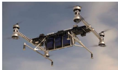
Fig. 9. The Boeing HorizonX is an unconventional eVTOL cargo air vehicle [32]
