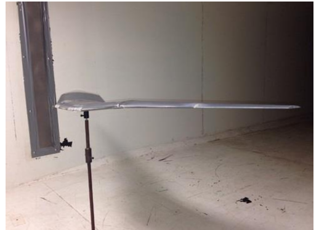
Fig. 14. Wing model used for application of Free Oscillation Method
