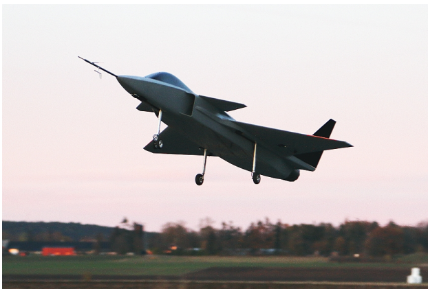
Fig. 3 The GFF demonstrator: a 2-meter, jet-powered platform used for research at Linköping University [22].
