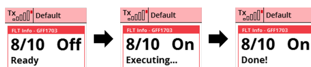
Fig. 6 Information window of the application during the execution of a test point, integrated on a transmitter Jeti Model DC-24.
