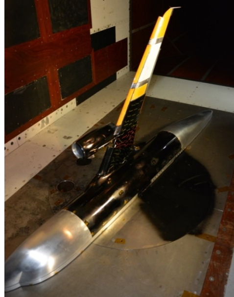
Fig. 6. HINVA High-Lift Model with slat cutout and AFC installed in DNW-KKK
