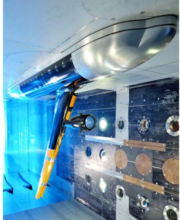
Fig. 2. HINVA model in ETW, taken with permission from [17].
