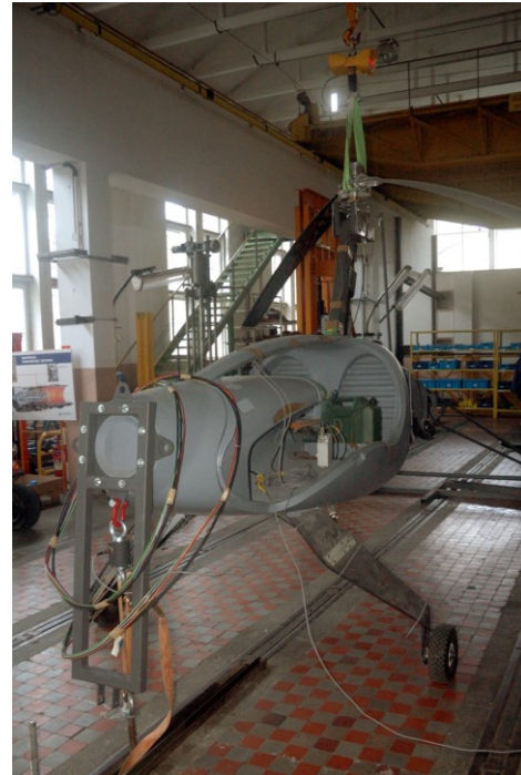
Figure 6. I-28A demonstrator during sensor calibration [IoA materials]
