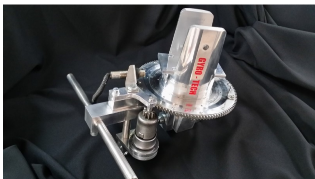
Figure 2. Rotor hub with pre-rotation and parking break
