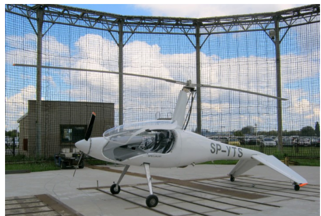
Figure 1. Autogyro I-28B in test rotors stand at the Institute of Aviation [IoA materials]
