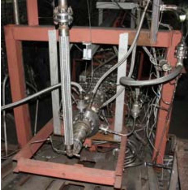
Figure 2. Experimental installation for the study of combustion processes in subsonic and supersonic quasi-air flows on a dynamometric platform. Components in the generator of high-enthalpy quasi-air flow are fed through flexible hoses perpendicular to the axis of the model combustion chamber.
