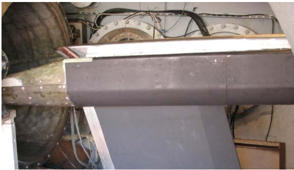
Figure 6. Scheme of large-scale model GLL-AP location on the CIAM test rig.
