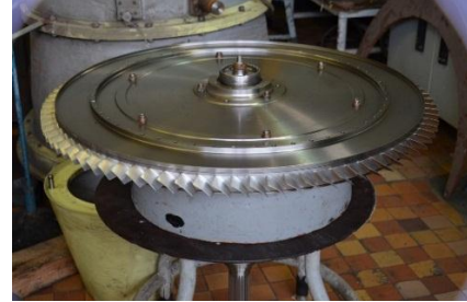
a) Rotor of the D-77M stage
