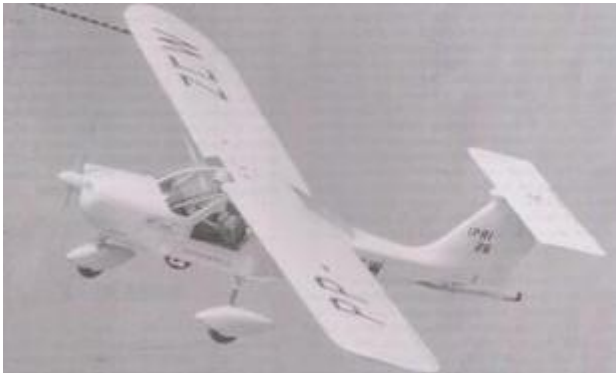
Fig. 18 The TUCA in flight, note the boom for the calibrated pitot and the tail stop parachute for the spin tests.
