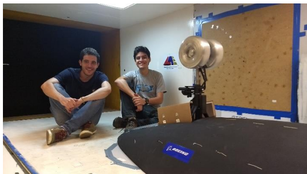
Fig. 23 Nose landing gear model tested at LAE-1 wind tunnel from Boeing BR&T project.
