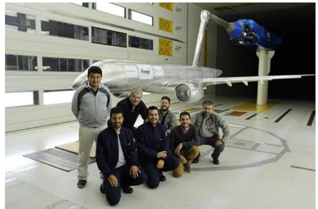
Fig. 212 Full model aeroacoustic testing at DNW ND. source author.
