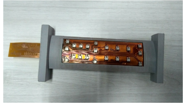
Fig. 5 Embedded circuit board mounted within the stator vane.
