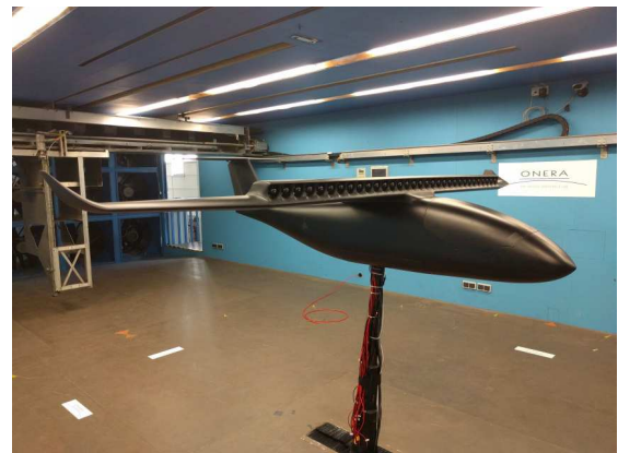
Fig. 3 The AMPERE scaled 1:5 model in ONERA's L2 wind-tunnel
