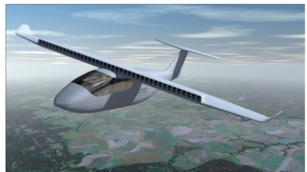
Fig. 2 AMPERE : High-wing concept plane with distributed Electric Ducted Fans EDF along the wing leading edge
