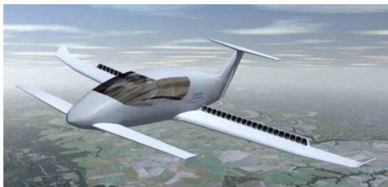
Fig. 1 Three-surface concept plane with distributed Electric Ducted Fans EDF at the wing trailing edge
