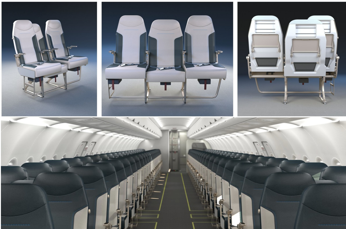
Fig. 4 Side-Slip Seat provides a wider aisle and enables a faster aircraft boarding: passengers could pass each other in the aisle or people with reduced mobility could easily reach their seat row ( https://www.airlineseats.biz/ ).
