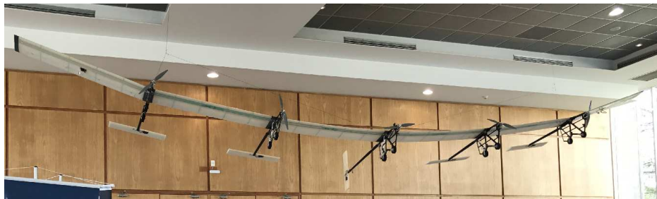
Fig. 1 – X-HALE aircraft hanging in the ceiling for concept demonstration. It was manufactured with built-in strain gages.
