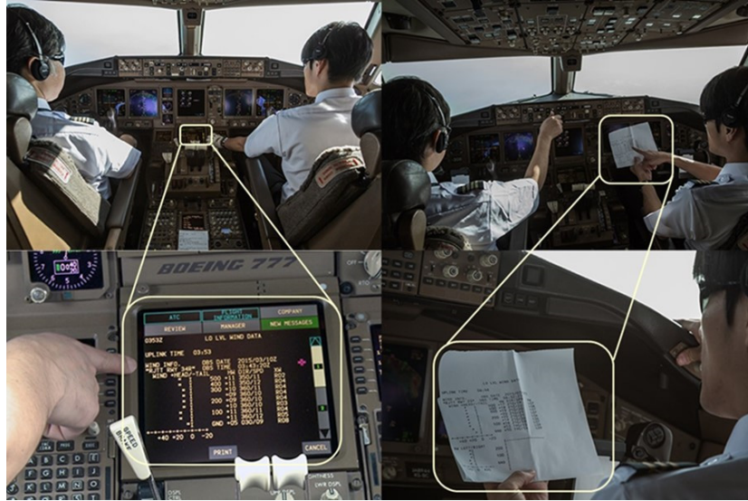
Figure 4. Use of ALWIN text display in the cockpit.
