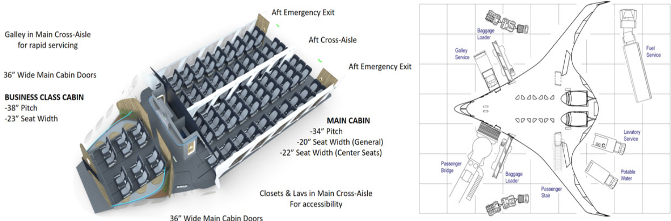
Figure 5. Ascent1000 cabin layout and ground servicing are conventional in many ways
