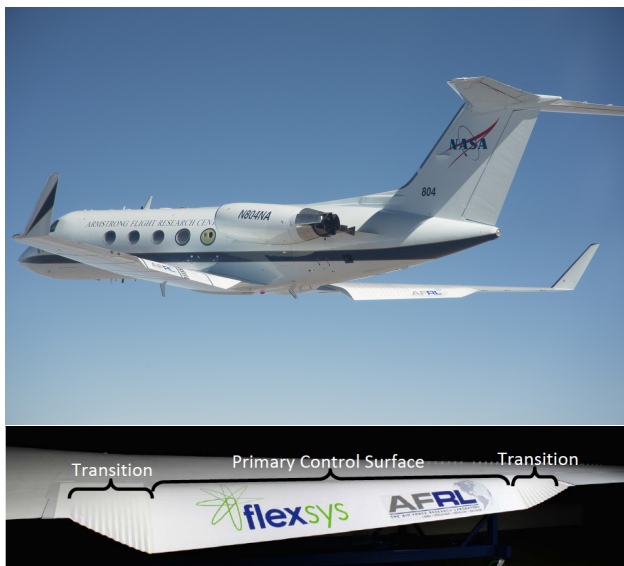
Fig. 1 High-lift flaps of a Gulfstream III business jet (NASA–Air Force test aircraft) were replaced with 19 ft multi-functional variable geometry control surfaces on each wing, including 2 ft wide transition surfaces.
