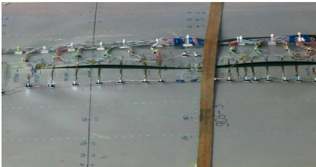
Fig. 8. Bulging of skin in full-scale fuselage with 2-bay longitudinal crack with broken stiffener
