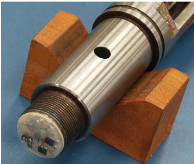
Fig. 4. A miniature, 50× gain, zero-drift, differential-output amplifier and its excitation-voltage regulator installed on the front face of a 44 mm wind tunnel balance
