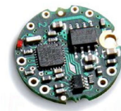
Fig. 5. Commercially available 20 mm dia. single-channel 24-bit digitizing and data transmitting module [6]
