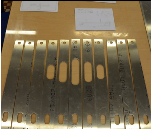
Fig. 14. Aluminum forms for gyroplane landing gear leg
