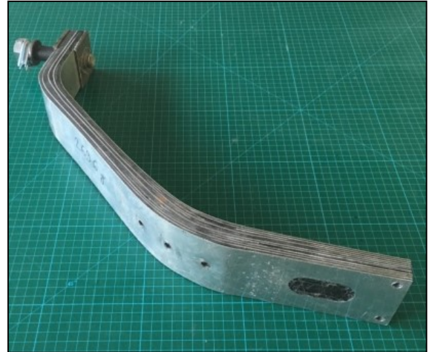
Fig. 17. Gyroplane landing gear leg prepared in hybrid technology
