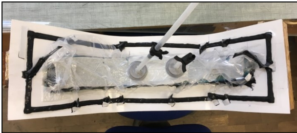
Fig.15. Gyroplane landing gear leg in a vacuum bag
