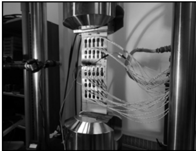
Fig. 4 Mechanical tests for CVM and LW systems installations
