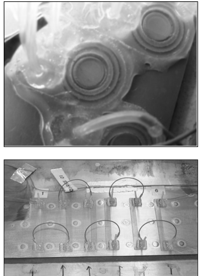
Fig. 1 Examples of CVM sensors installed in a metallic R&D barrel test and in the E-Jets Full-Scale Fatigue test
