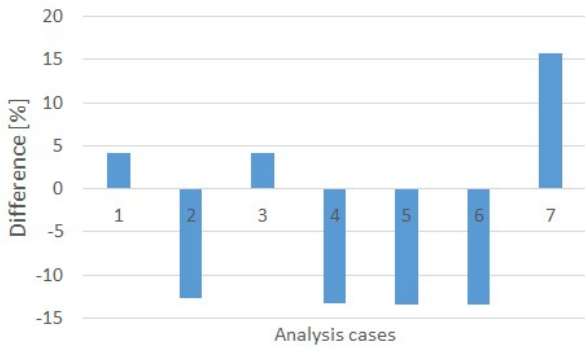
Figure 10 – Delamination onset when using default tolerance and an initial increment 0.05.
