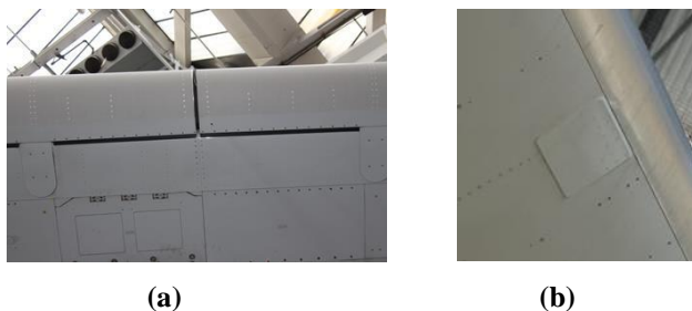
Fig. 7 Wing excrescences: gaps associated with moveable surfaces (a) and repair patch (b)
