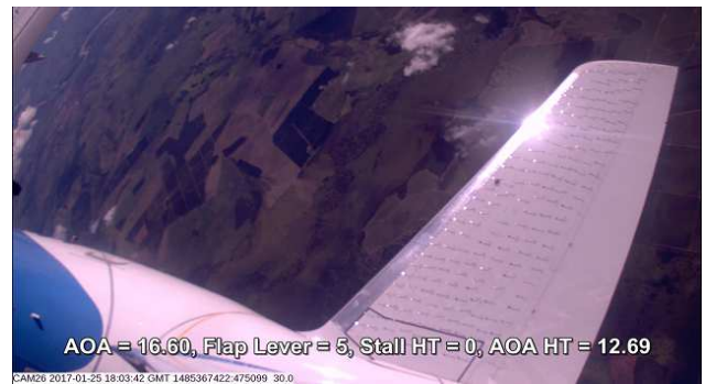
Fig 12 – Tufts flow visualization combined with HT measurements during a high incidence flight-test maneuver
