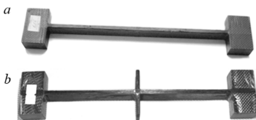
Fig. 1. Photo of the specimens: (a) - “rib”, (b) - “rib crossing”.
